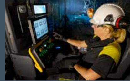
RCS-based carrier control system with logging and reporting functions means easier and faster maintenance and an enabler for tramming automation.
